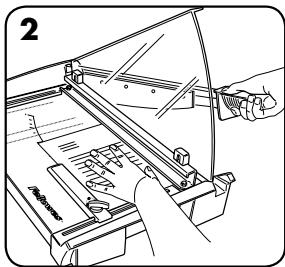
2. Hold paper with hand and / or clamping mechanism to ensure it doesn't move while trimming. Make sure that hands are not under the blade.
