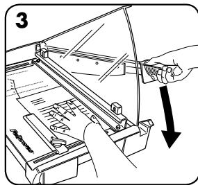
3. Push handle downwards in a continuous motion.
