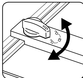
Rotate knob to lock and unlock the edge guide.
