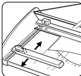
For adjustment as required, turn locking lever to (🔓). To lock, turn locking lever to (🔒).
