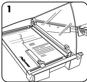
1. Place item (e.g. photo or paper) onto cutting table. Align paper with markings on the base of the trimmer.
