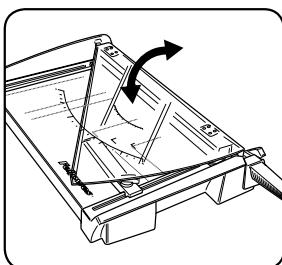
The SafeCut™ Guard is folded down for transport and storage – it also holds the handle down to avoid injury risk. Folded up the SafeCut™ Guard guides the cutting bar/blade lever and ensures user can't harm themselves with the blade when cutting. *Do not attempt to put your hand under the cutting bar or touch the blade.*
